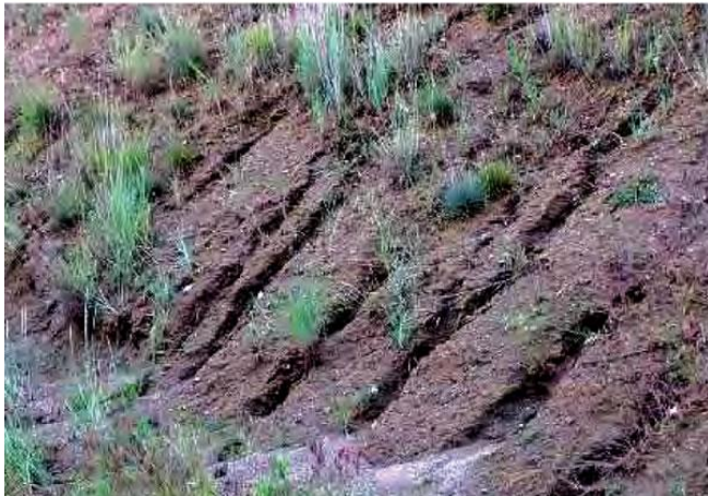
Highway slope stabilization research in Washington State evaluated compost's performance for erosion control and vegetation establishment (with compost (top) and no compost (below))
