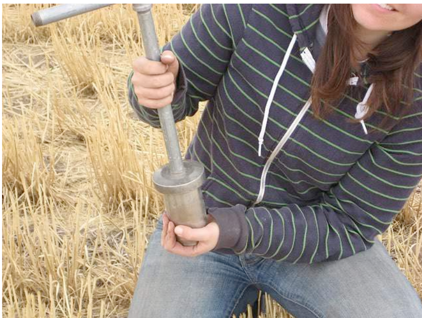
Collecting bulk density sample in 3 dry ton/acre biosolids treatment
